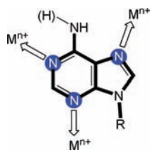
FIGURE 1. Chemical structure of adenine (imino nitrogens important for metal ion coordination are highlighted). The exocyclic amino group may coordinate via deprotonation.
